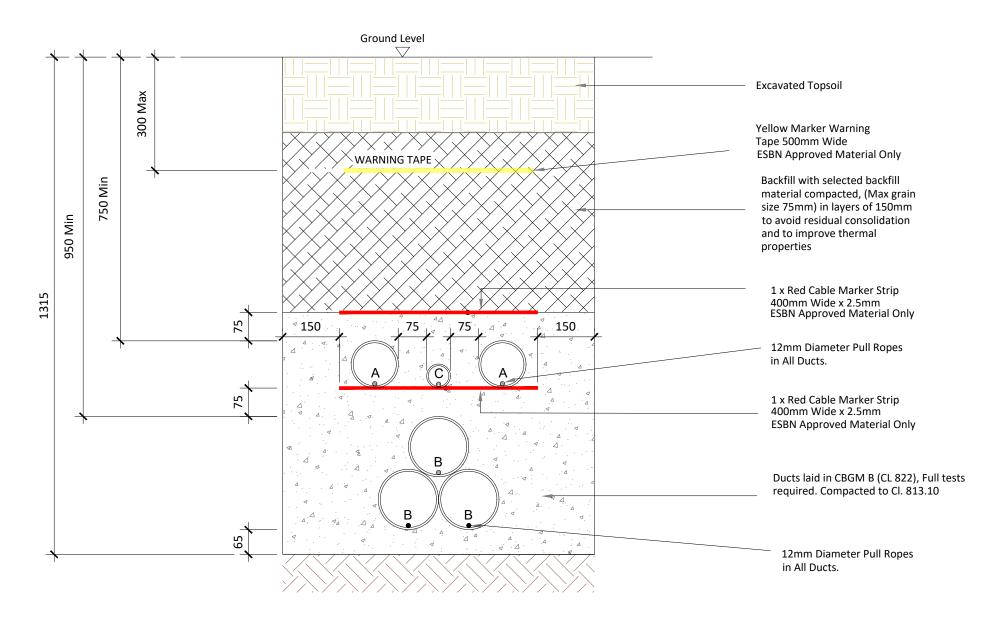
A = 125mm: Outer Diameter HDPE ESB Approved Duct, SDR=17.6 B= 160mm: Outer Diameter HDPE ESB Approved Duct, SDR= 21 C = 63mm: ECC Earth Continuity Conductor
